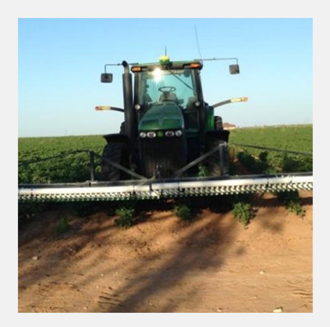
The pressure vacuum recirculating system includes a 12-volt pump, which delivers a constant flow of herbicide to the rope. This produces a more even application of the herbicide and minimizes drip from the rope onto crop plants. It also allows recovery of any unused herbicide, so it minimizes waste.
